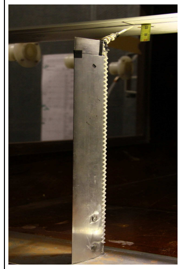
(b) Hot wire mounted in wind tunnel, from [193].
