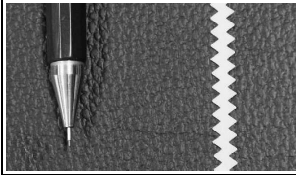
Figure 6.4: Zig-zag tape used for tripping the boundary layer on the airfoil, from [193].
